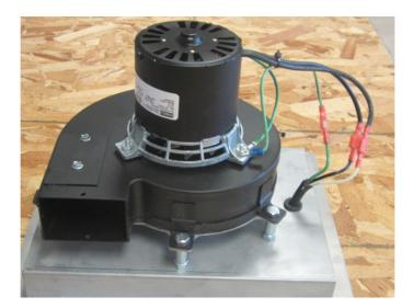
This is the fan and motor assembly attached to the mounting plate and fastened over the stainless steel thimble face on the outside wall of the house. This is the same fan and motor assembly we have been using on our other conversion kits for the last 4 years.
