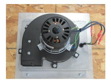
The fan and motor assembly can now be mounted to the mounting bracket. Again, the bracket will fit over the stainless steel brackets and must be centered side to side. After the bracket is centered, mark the mounting bracket holes on the stainless steel thimble face and use a small pilot drill bit to make your mounting holes. Included are #10 X 1" screws. You may need longer ones depending on the material on the side of the house.
