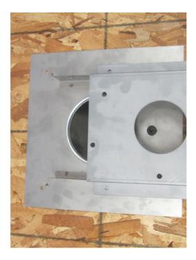
This is the mounting plate without the fan and motor, slid off to the side. The mounting plate fits over the angle pieces of stainless steel. The plate will have to be centered left to right on the face of the thimble to insure the exhaust tube is centered inside the fresh air intake tube.
